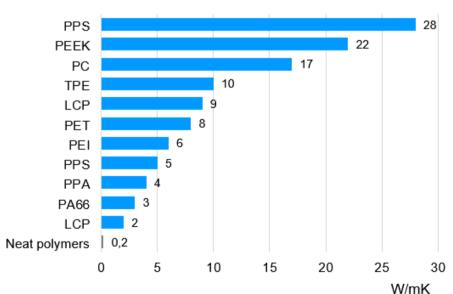
Up to 200 times higher thermal conductivity with LUVOCOM TC. Examples based on various polymers
