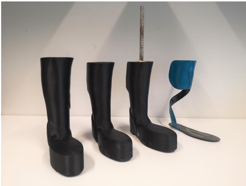
3D printed molds, finished CFRP orthotic
