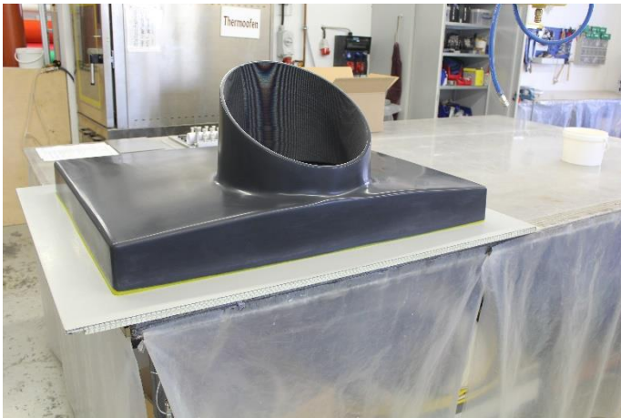
Stage 2: Condition after surface fillers were applied
