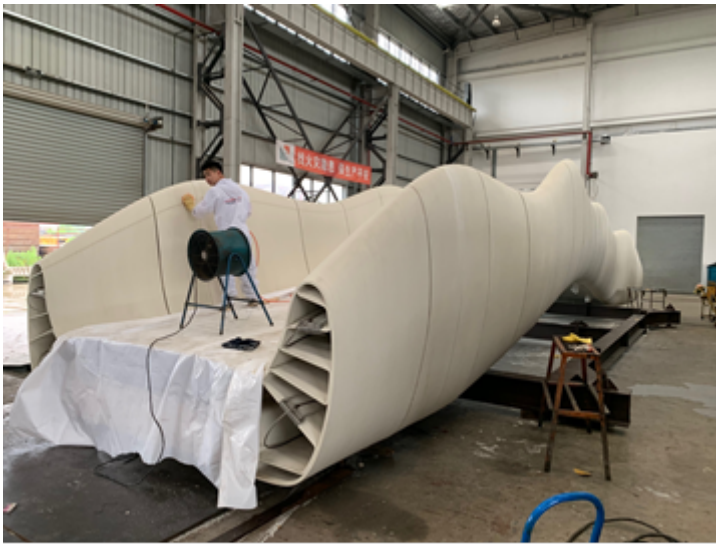
Think Big! FGF-printed bridge component in China.
