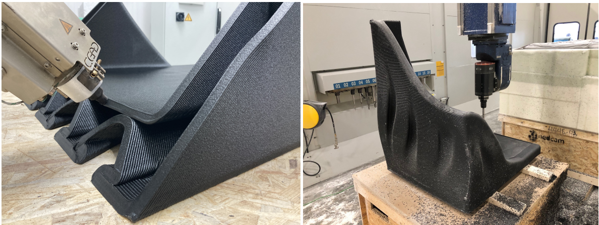
FGF-compliant design and creation of the final contour by milling (courtesy of Nedcam Solutions B.V.)
