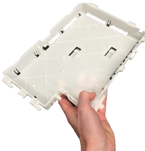
Printed to match injection molded - printed spare part for a dishwasher does not allow 3D printing-specific adaptation of the geometry, here LUVOSINT PP 8824 WT.
