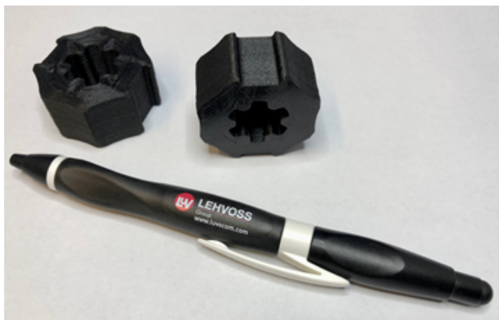
Precise FGF printing: LUVOCOM 3F PAHT 9742 CF printed on Pollin AM Series P-HT (courtesy of Pollen AM Inc.)
