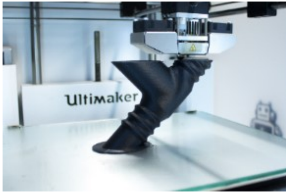
Photo: High-performance fiber-reinforced materials run on technically simple, cost-effective filament printers
