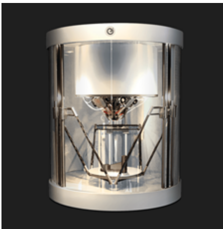
Precise FGF printing: LUVOCOM 3F PAHT 9742 CF printed on Pollin AM Series P-HT (courtesy of Pollen AM Inc.)
