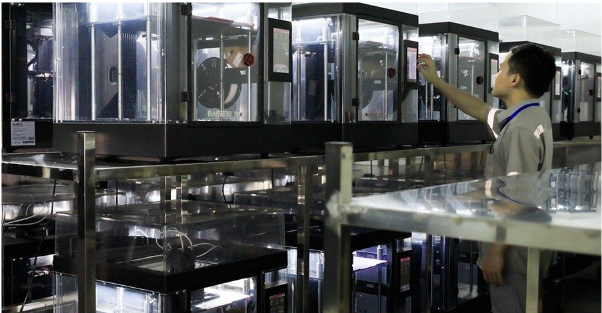
200-printer farm, China, managed by two operators only (courtesy of Raise3D)
